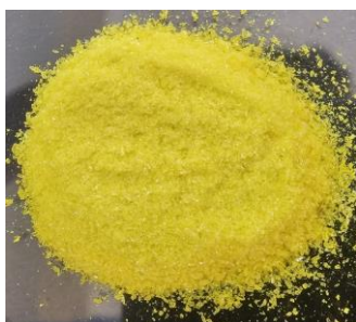
Figure 2. Macroscopic morphology of FOX-7 crystals.
