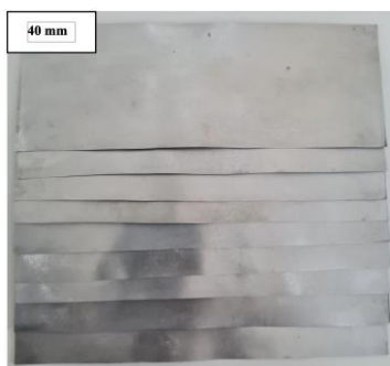
Figure 1. FeCo49V2Nb0.2 alloy plate after fabrication.
