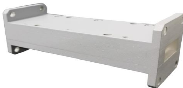
Figure 6. The fabricated harmonic filter.
