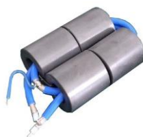
Figure 7. Power matching transformer T2.
