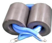
Figure 6. Power combiner transformer T1.
