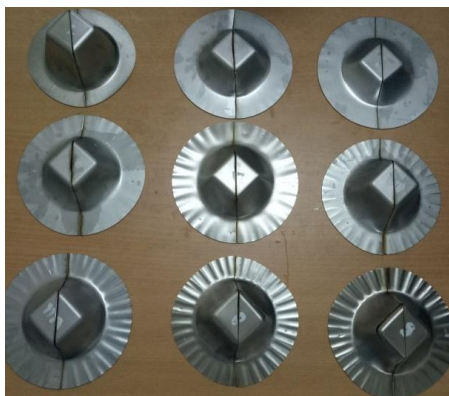
Figure 3. The formed square conical parts obtained from the experiments.
