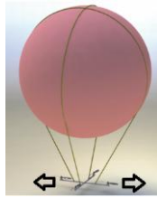
Figure 9a. Concept of suspending a drone with a flexible wire under the balloon body (Italy, 2017).
