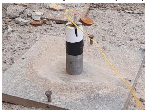
Figure 4. Lead cylinder before compression testing.
