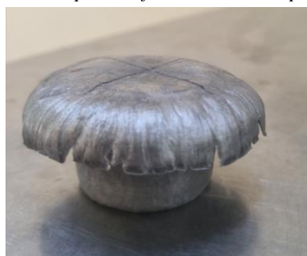
Figure 5. Lead cylinder after compression testing.
