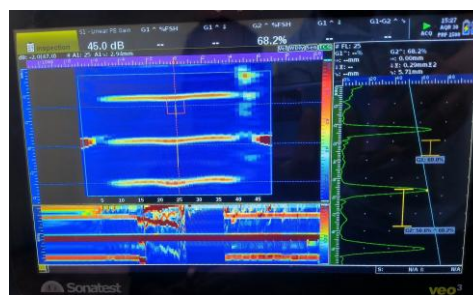
Figure 5. Ultrasonic defect inspection.
