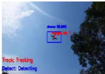
c) Drone detecting and tracking in strong light and closed trees condition.
