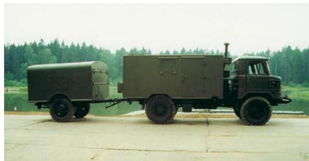
Figure 1. VFS-2.5 water filtration station in marching condition.
