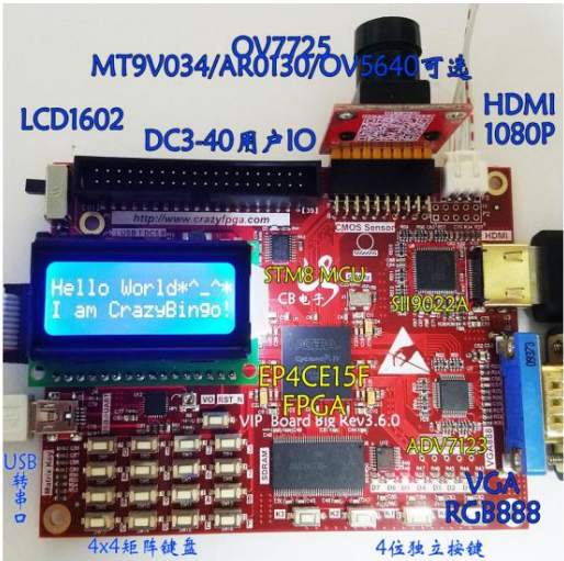
Figure 1. The VIP Board Big V3.8 with Cyclone IV FPGA and peripheral interfaces.
