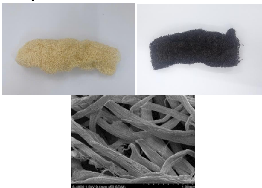
Figure 5. CDs/luffa composites and SEM image.
