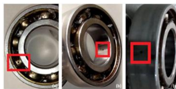
Figure 1. Defected bearings with different faults: (a) Ball, (b) Inner race, (c) Outer race [8].
