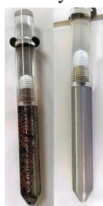
Figure 2. Rust resistance test according to ASTM D665.
