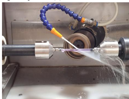
Figure 4. Cylindrical grinding process of the glass laser rod.
