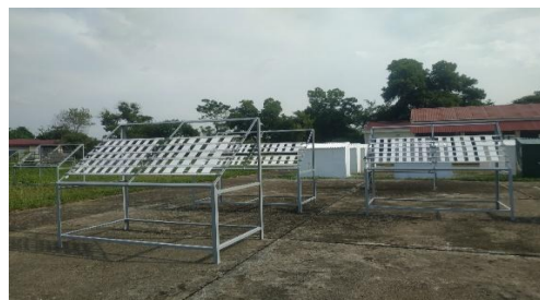
Figure 2. Drying racks for heat reflective paint samples on concrete floors.
