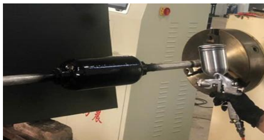
Figure 6. Manufacturing of the sealing layer.
