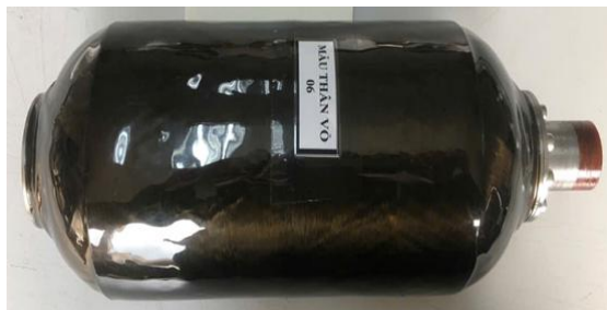
Figure 7. Composite SRM after winding.
