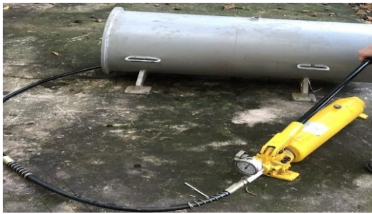
Figure 8. Pressure strength testing of the SRM without propellant.
