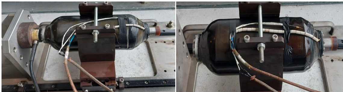
Figure 10. Composite SRM casing before and after the firing test.
