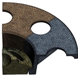
Figure 1. Quarter-symmetry finite element mesh model of the original baseplate.
