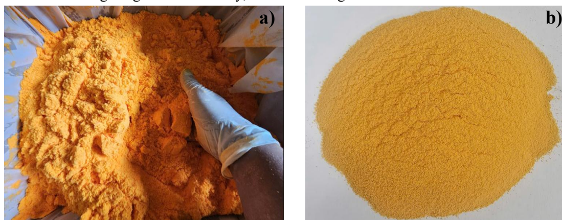
Figure 1. Morphological appearance of the synthesized A-IX-1O explosive: (a) post-filtration; (b) post-drying.
