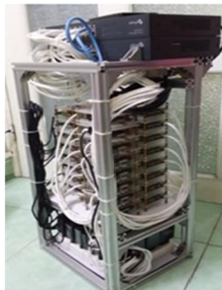
Figure 1. Raspberry Pi 3 B+ cluster 24 nodes.
