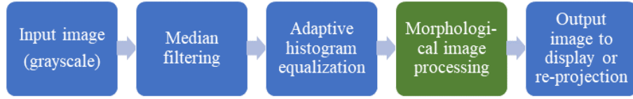
Figure 3. Diagram of our image processing procedures employed morphological image processing to enhance vein image.
