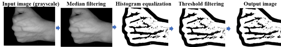
Figure 4. Vein image of a human's upper hand after typical image processing procedures, showing hairs remain and affect output images.
