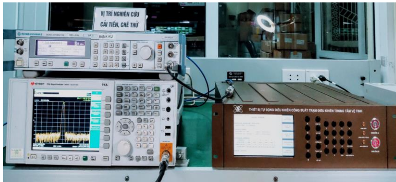
Figure 8. Actual test connection of the UPC.
