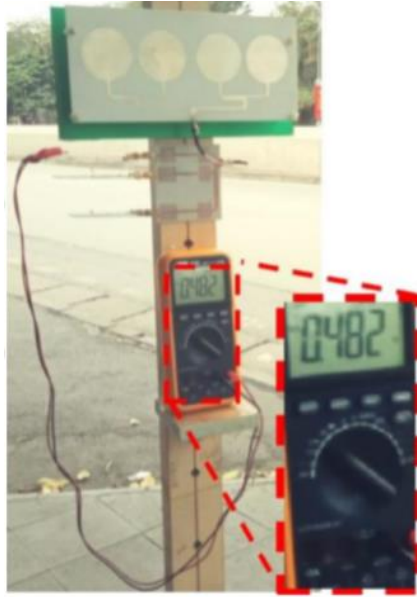
Figure 6. The antenna array inside a rectenna in the ambience.
