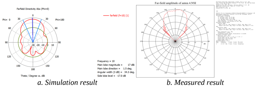
Fig. 9. Radiation patterns in the elevation angle at a frequency of 10 GHz.
