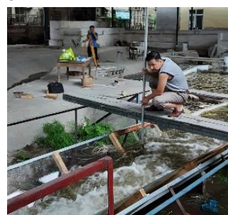
Figure 7. Measuring water level data by a leveling staff.
