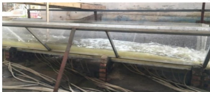
Figure 6. Hydraulic jump in trapezoidal channel (side slope 1:1) with Q = 118 l/s and Fr_1 = 4.19 .
