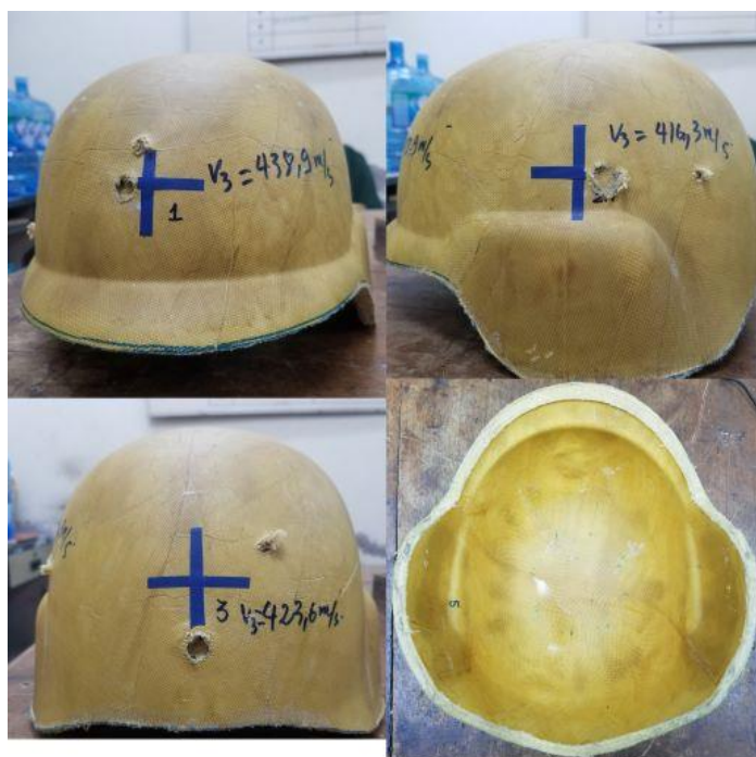
Figure 6. Images of ballistic resistance of composites in the shape of the helmet.
