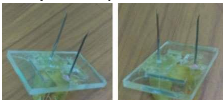
Figure 6. Electrodes using for measurement the impedance of pork meat.
