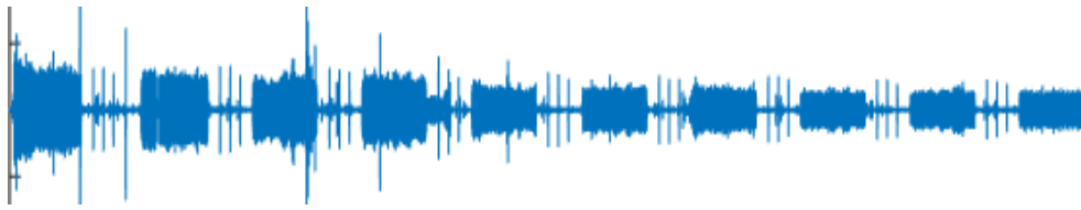
Figure 10. 10 OFDM received Frames.
