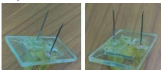
Figure 4. Electrodes are used to measure the impedance of pork meat.
