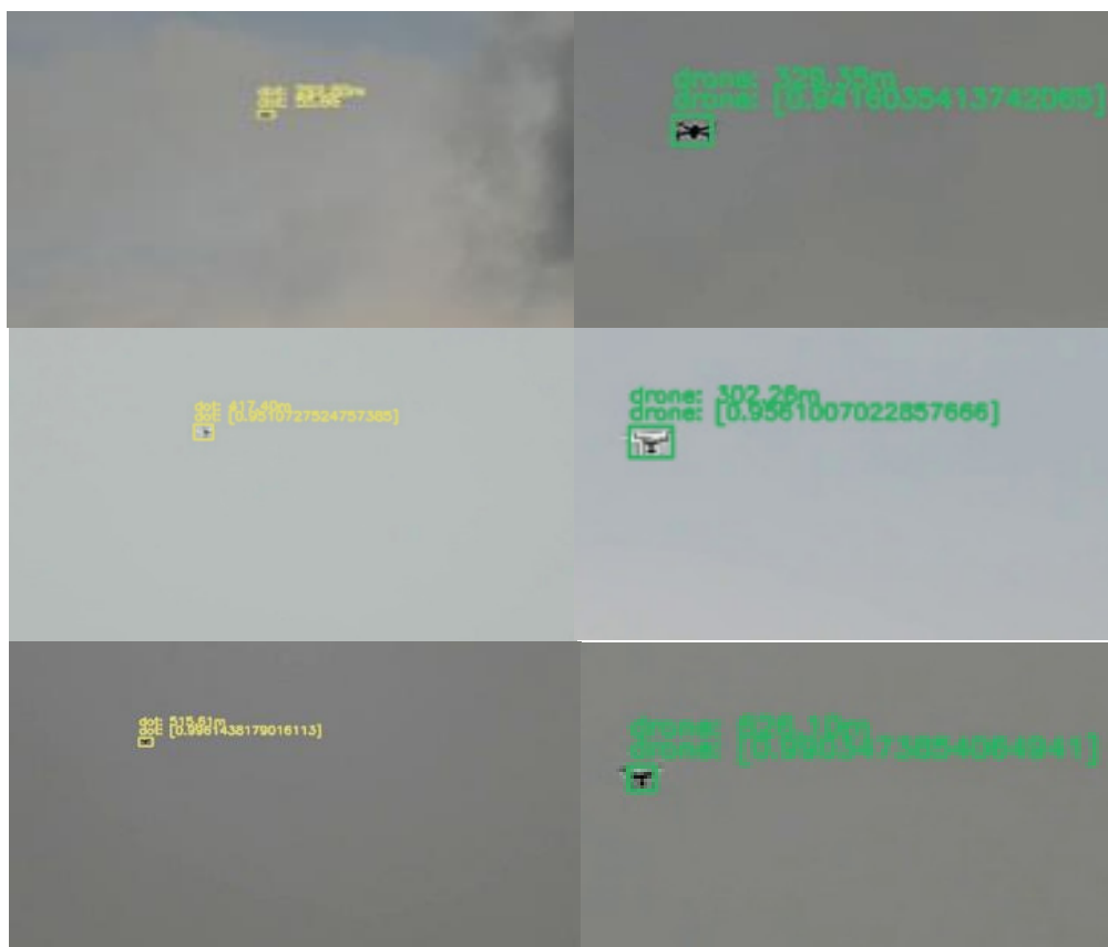
Figure 10. System found a dot (left) and then verify it is a drone (right).
