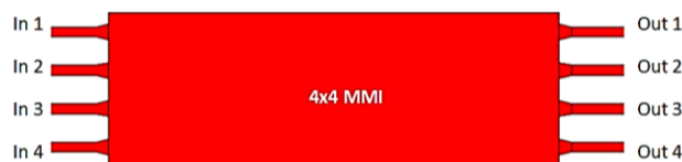
Figure 1. The structure of the DST and DCT using a 4x4 MMI coupler.
