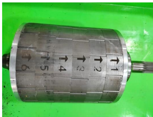
Figure 13. Rotor lamination with six step-V shape skew magnet slices assembly.
