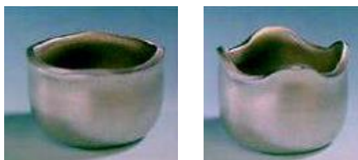
Isotropic material Anisotropic material Figure 1. Products of the deep drawing process.
