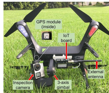
Figure 2. 3DR Solo quadcopter retrofitted.
