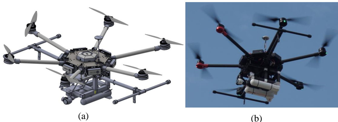
Figure 1. (a) (b) Mounting design of the ammunition on the bracket of the drone.
