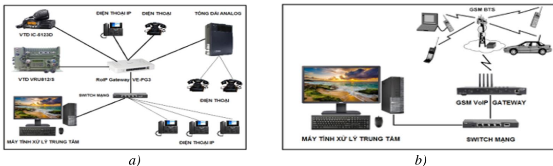
Figure 1. Communication diagram of RT (a) and GSM (b) connection blocks in the system.
